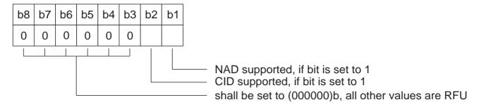
Figure 8 — Coding of interface byte TC(1)
