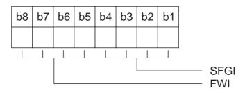
Figure 7 — Coding of interface byte TA(1)
