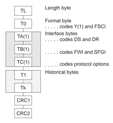
Figure 4 — Structure of the ATS
