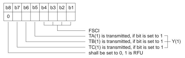
Figure 5 — Coding of format byte
