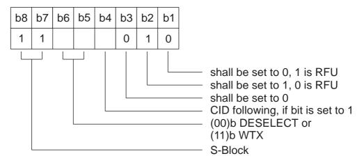
Figure 17 — Coding of S-block PCB
