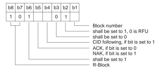
Figure 16 — Coding of R-block PCB
