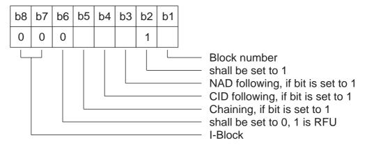
Figure 15 — Coding of I-block PCB
