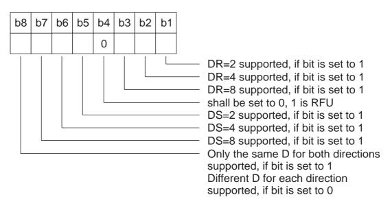
Figure 6 — Coding of interface byte TA(1)
