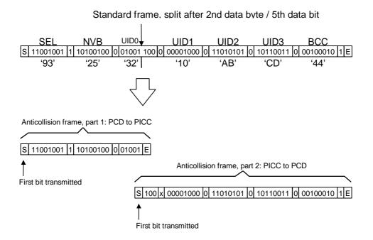
Figure 6.5 – Bit organization and transmission of bit oriented anticollision frame, case SPLIT BYTE
