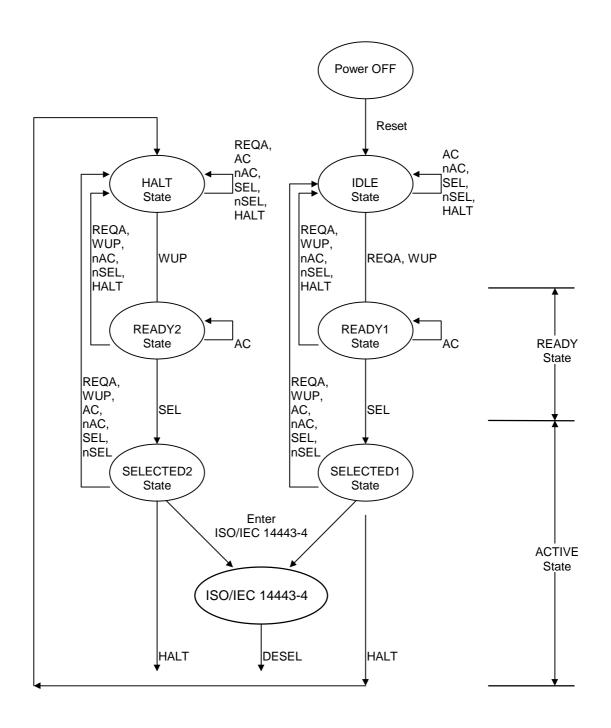
Figure D1 - Detailed PICC Type A state diagram
