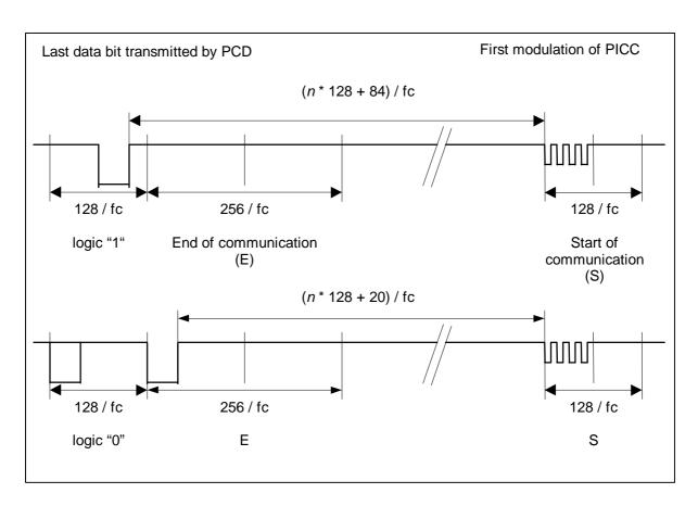
Figure 6.1 - Frame delay time PICC to PCD
