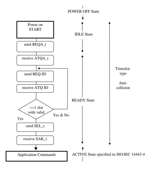
Figure C1 - Flow chart of Timeslot-type Anticollision
