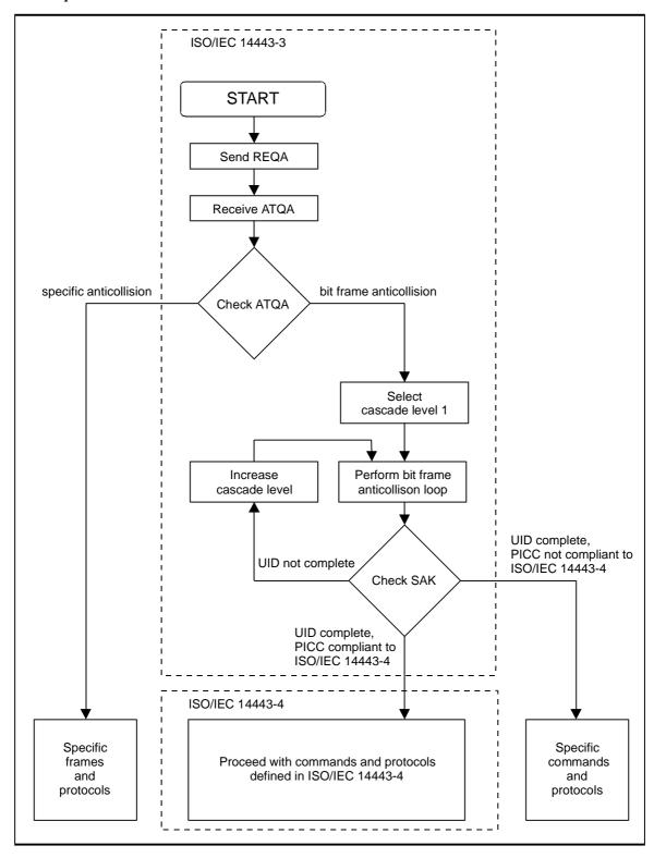
Figure 6.8 – Initialization and anticollision flow-chart for PCD
