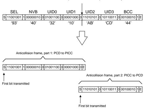
Figure 6.4 - Bit organization and transmission of bit oriented anticollision frame, case FULL BYTE
