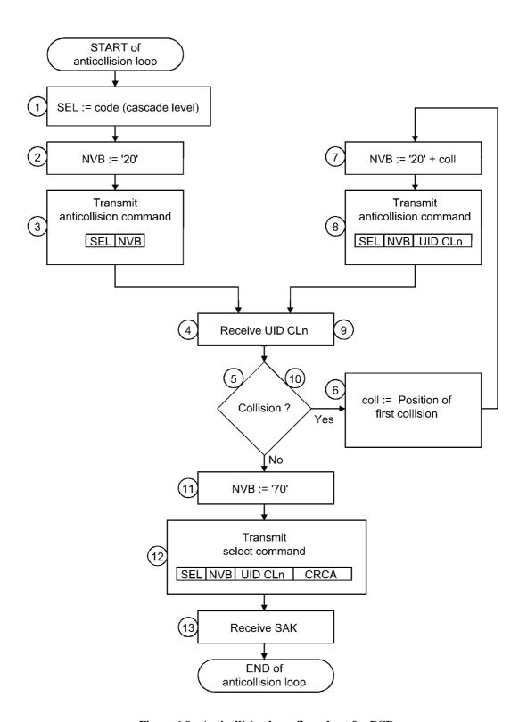
Figure 6.9 - Anticollision loop, flow chart for PCD
